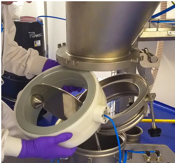
J-Tec quick clean dosing valve that is easy to disassemble
